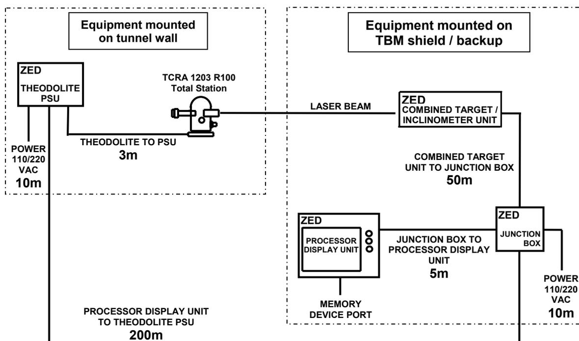
An important advantage of having this type of equipment is to greatly reduce the downtime when repositioning the laser station, For example, Morgan-Est (formerly Miller Civil Engineering), a UK contractor working on a sewer project in Hull, in the UK, with forward planning, were able to reposition the instrument in less than 30 minutes; basically the time required to physically move the total station and rearrange the cabling.
